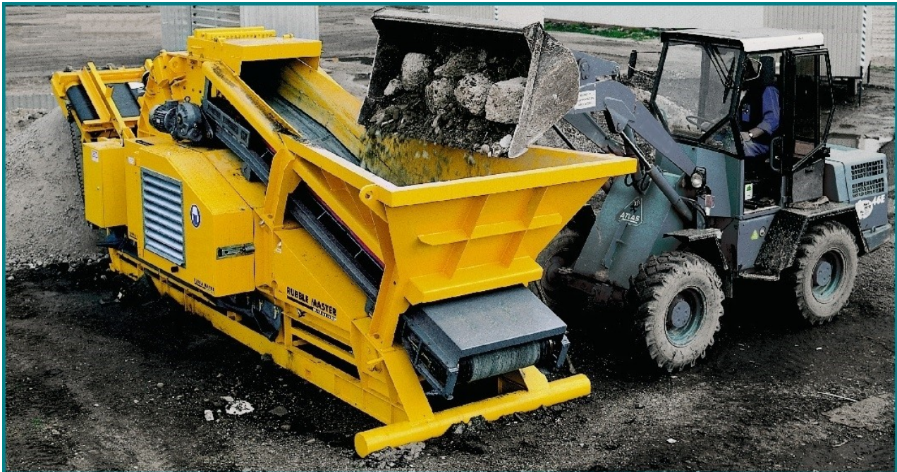
Figure 10: Example: Mobile concrete crusher RM 60 by Rubble Master
